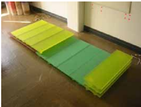
Material: Acid washed laminated water white glass, 48" x 16" x 2" each element.
